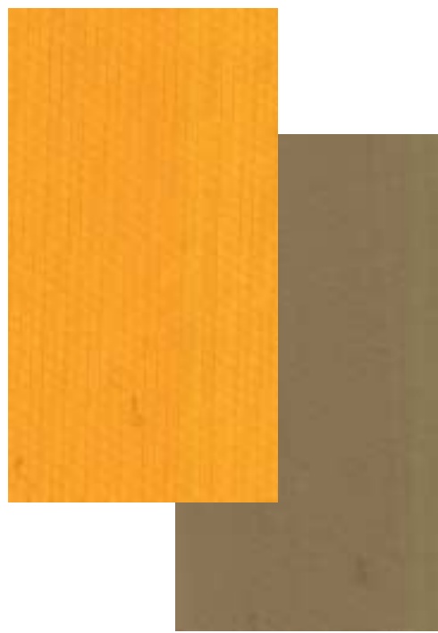
Above: Face and back of a new lightweight waterproof/breathable fabric developed by Middendorf in partnership with the filtration company Tetratex. It is a 3-ply laminate of ripstop/PTFE/tricot. Weight: 3.1 ounces/yd.
